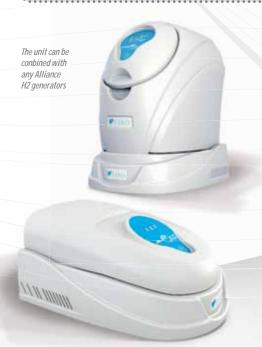
**ZERO AIR WITHOUT INTEGRATED COMPRESSOR**: produces dry and hydrocarbon-free air < 0.05 ppm, using a heated catalytic technology and connecting it to a dry compressed air supply. Allows to be used individually or coupled to any one of the F-DGSi H2 generator to form an all-in-one FID gas station solution.
