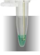
Injection of an ice crystal by cooled triggering needle (cryst-needle).
