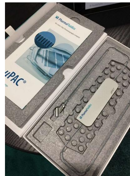
To serve your custom separation needs,  $\mu$ PAC<sup>®</sup> cartridges are available in various lengths and equipped with connectors matching your application. Stationary phase chemistry is currently focusing on reversed phase HPLC separations.
