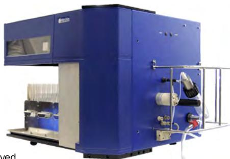
The automatic gain adjustment ensures that peaks will be resolved without signal saturation (flat top peaks). The fume enclosure option permits bench-top installation, outside of a fume hood.
